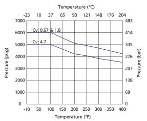
The pressure rating of CH Series check valve is restricted by the connection types. For details please refer to B-148.
