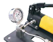
Fig. 7 Pressurize to the Pressure Specified in Table 1
