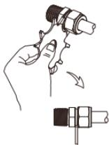
If the gauge will not enter the gap the fitting is sufficiently tightened
