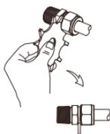
If the gauge will enter the gap additional tightening is required
