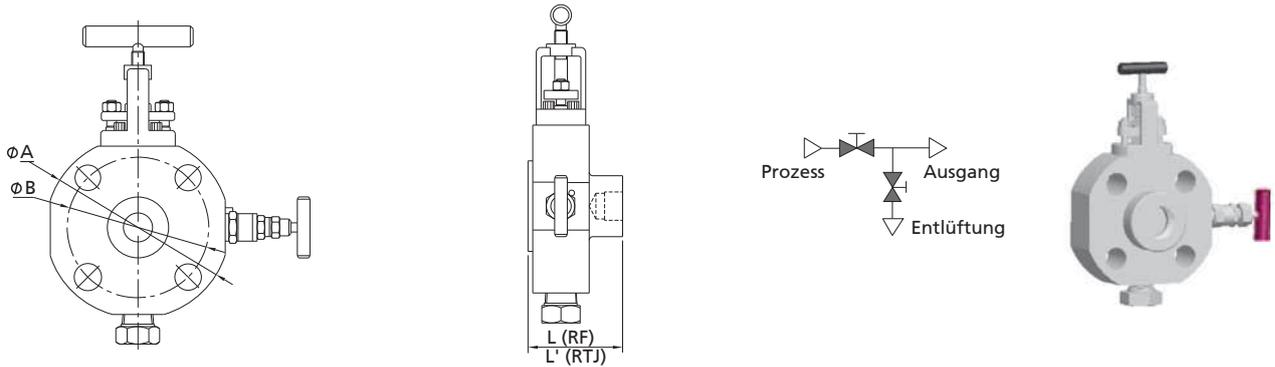
Absperr: Nadel    Ablass: Nadel    (Konfiguration: NN)
